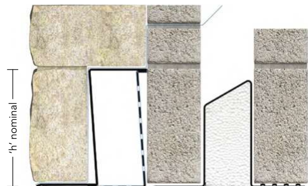
BOX/K-200 lintel shown with optional feature plate.
