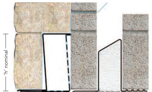
BOX/K-200 lintel shown with optional feature plate.
