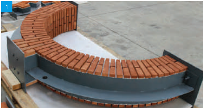
1 Segmental Arch with Keystone in production
