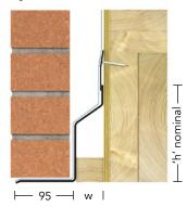
T/K-70 W = 68mm - for 70 to 85mm cavity widths T/K-90 W = 88mm - for 90 to 105mm cavity widths
