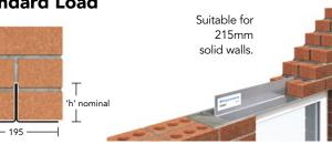
To achieve loading figures lintel must be built in as shown. Lintels may be propped to facilitate speed of construction. See Lintel Installation on page 6.
