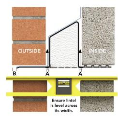
In accordance with BS EN 1996-2:2006 and NHBC requirements all external wall lintels MUST be installed with a flexible damp proof course with the exception of those adequately protected by an eaves overhang or similar form of protection.
