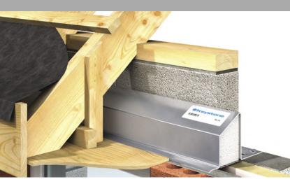
EL/K lintels are designed to provide support over openings at eaves level. The eaves lintel has a shortened outer flange to allow the underside of the soffit board to be positioned tight against the window frame. It must be noted that brickwork cannot be built onto the outer flange of an eaves lintels. Masonry is built on the inner leaf only.
