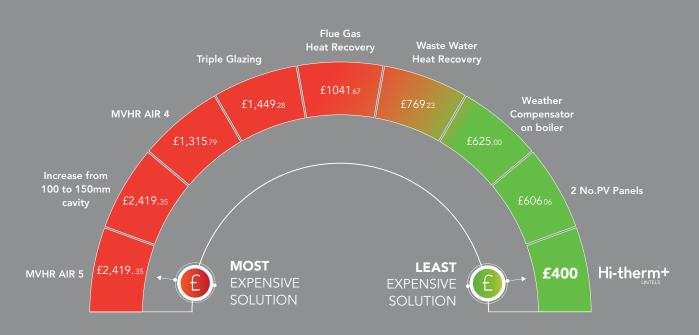
This case study is based on an actual semi detached 75m<sup>2</sup>, 3 bedroom house design and the figures were produced by an independent energy assessor using SAP 2012 software.
