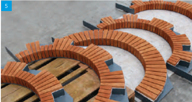
4 Bullseye Arch 5 Keyslip Brick Feature Lintels in production 6 Brick Slip Apex Arch
