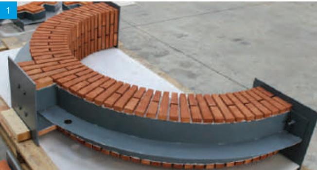
1 Segmental Arch with Keystone in production 2 Perforated steel lintel 3 Bricks are bonded to steel lintel in factory controlled environment
