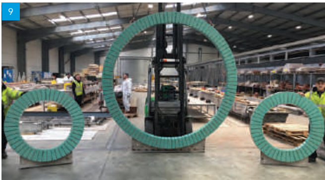
7 Bullseye Brick Feature Lintel 8 Precision cut bricks applied to steel lintel 9 Bullseye Arches with glazed bricks
