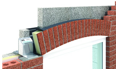
Diagram 4 - Section through Product installed in a typical masonry cavity wall (cavity tray below the Product)
